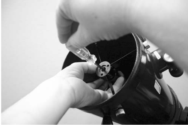
Figure 11. To center the secondary mirror under the focuser, hold the secondary mirror holder in place with your fingers while adjusting the center screw with a Phillips head screwdriver. Do not touch the mirror's surface.
