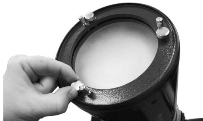
Figure 14. The tilt of the primary mirror is adjusted by turning one or more of the three wide collimation thumbscrews.
