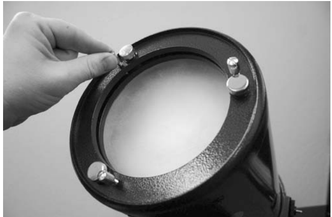
Figure 13. The three thin thumbscrews that lock the primary mirror in place must first be loosened before any adjustments can be made.
