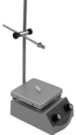
Screw the two rods together, creating one support rod. Make sure they fit tightly. Insert the slotted end of the rod into the plastic holder on the back of the base. Slip the right angle clamp onto the support rod and tighten the knob. Slide in the thermometer holder and tighten the other knob. The height of the thermometer holder can be adjusted by moving the clamp up or down on the support.
