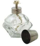
Assemble your lamp by removing the wick from the glass body (a bent paperclip will do this easily) and inserting it through the hole in the cap. The wick should protrude about 3/8" from the top of the metal cap. Spread out the wick fibers similar to the photo.
