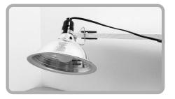
Your student may need a box or stack of books to set the experiment at the right height next to the light bulb. This will depend on the height of the heat lamp. Each bottle should be about 5 cm away from the bulb.
