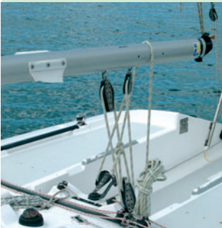
The more pulleys in a pulley-block, the less force needed to move the load.
