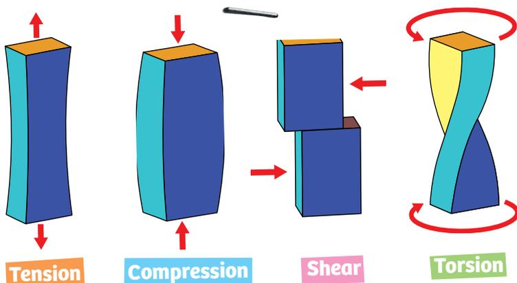
Structural engineers often use four terms to describe how a load can affect a structure: tension, compression, shear, and torsion.
