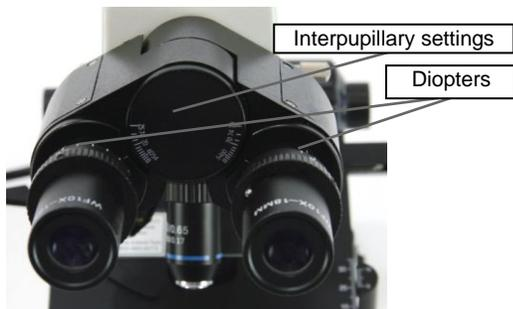
4. Open or close the distance between the eyepieces by pulling them apart or pushing them together until the two circles merge together and appear as one circle. The interpupillary distance is set correctly when you see just one field view circle. Record the settings so you can return to your adjustment easily.
