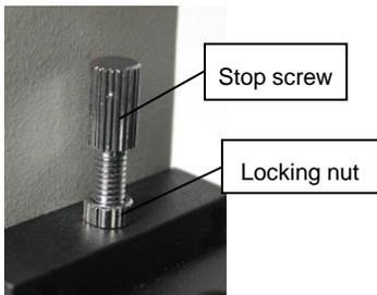
**Note:** The higher the stop screw position, the higher the stage will rise.
