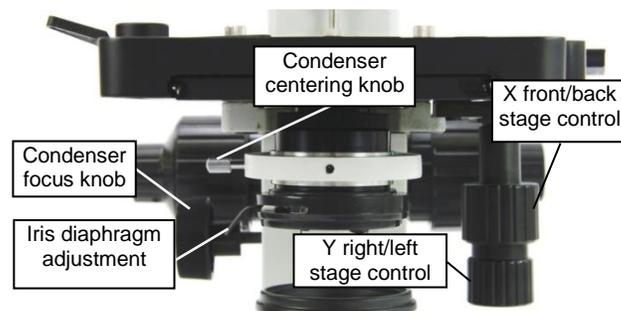
9. **Iris diaphragm:** The diaphragm controls the amount of light coming through the specimen in order to provide the best contrast for the objective lens. It is fully adjustable by moving the lever below the stage. Generally, you need less light on lower power and more light on higher power.
