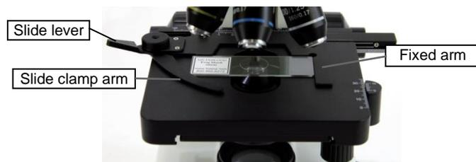
5. Move the small lever on top of the stage to open the curved slide clamp arm.
