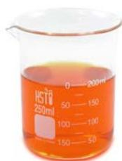
**Griffin beakers** are used to mix chemicals, dissolve into solutions, heat or cool solutions, and hold sand or water baths. They typically have graduations, but they are not very accurate.
