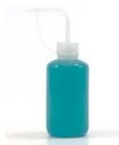
**Wash bottles** are plastic bottles with a nozzle at the top for rinsing glassware, cleaning/disinfecting, or applying solutions. They can be filled with a variety of reagents, such as water or alcohol.
