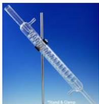
**Condensers** are used to condense chemical vapor into a liquid. This is done by sending the vapor through a long (often coiled) glass tube to cool.
