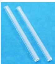
**Glass tubing** is usually inserted into stoppers to attach rubber tubing, but it can also be used to splice two pieces of rubber tubing. It can be cut with a file or tubing cutter and shaped with a flame.
