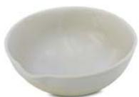
**Evaporating dishes** are used to separate water and solids from a solution by allowing the water to evaporate off into the air. This is usually done by heating the evaporating dish over a burner.
