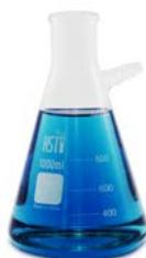
**Filtrating flasks** are used to filter mixtures through a funnel and filter paper. A tube near the top prevents unwanted pressure buildup. The process can be accelerated with a vacuum pump.
