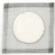
**Wire gauze** is a fine mesh wire sheet that is used to evenly distribute heat from an open flame. It rests on a support ring attached to a ring stand and holds glassware above a burner.
