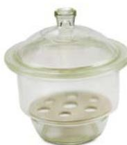
**Desiccators** are sealable containers for low-humidity and dust-free storage. The most common type is round, made of heavy glass, and has a removable platform inside. Desiccant sits below the platform and items to be stored sit atop it.
