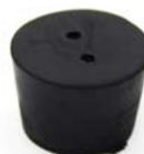
**Stoppers** are used to seal narrow-mouth containers such as flasks and test tubes, and to hold pieces of glass tubing for distillation experiments, or to mount thermometers inside a flask.
