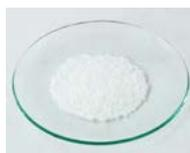
**Watch glasses** can be used to cover beakers, evaporate water from solutions, weigh out solid chemicals, or observe samples under a stereo microscope.
