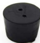
**Stoppers** are used to seal narrow-mouth containers such as flasks and test tubes, and to hold pieces of glass tubing for distillation experiments, or to mount thermometers inside a flask.
