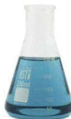
**Erlenmeyer flasks**, like beakers, can be used to mix, dissolve into solutions, and heat or cool solutions. In addition, they can be plugged with stoppers and used to catch vapor or condensed liquid. Graduations are not very accurate.
