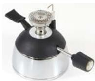
**Lab burners** come in many different styles and usually run on alcohol, propane, or butane. They are used to heat or boil solutions, burn or melt solid chemicals, or form glass tubing.
