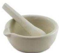
A **mortar and pestle** is used to crush up solid chemicals into smaller pieces, or to grind solids into fine powder. This makes dissolving solids into solutions much easier.
