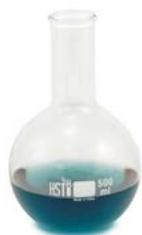
**Florence/boiling flasks** are round to provide uniform heating or boiling of liquids. They can be used to mix or store solutions as well as collect vapor in distillation processes. They can have either round or flat bottoms.
