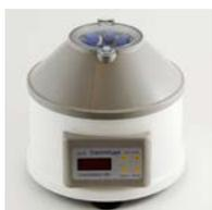
A **centrifuge** is a motorized device used to spin liquids at high speeds. In labs, a centrifuge uses gravity and centrifugal force to separate substances with different mass. An example is separating particles from a liquid.
