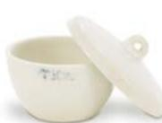
**Crucibles** are used to melt or burn solid chemicals over a burner. They are made from heat-resistant ceramics to prevent breakage.
