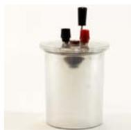
A **calorimeter** measures the heat transfer during a chemical reaction or physical change. A reactant is placed inside the inner chamber of the calorimeter. Measuring the temperature difference before and after allows heat transfer evaluation.
