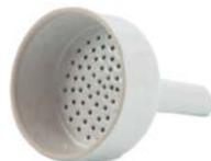
**Funnels** are used to pour liquids into narrow-mouth containers such as flasks and bottles. **Buchner funnels** (pictured) are special two-piece funnels for filtering mixtures through filter paper into a filtering flask.
