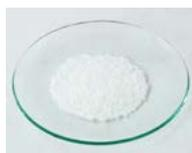
**Watch glasses** can be used to cover beakers, evaporate water from solutions, weigh out solid chemicals, or observe samples under a stereo microscope.
