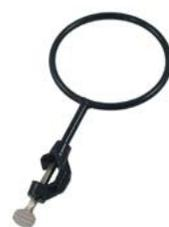
**Ring supports** are also called iron rings or ring clamps. Used with a ring stand; ring supports raise and secure an object above a work surface. For example, a round bottom flask or separatory funnel.
