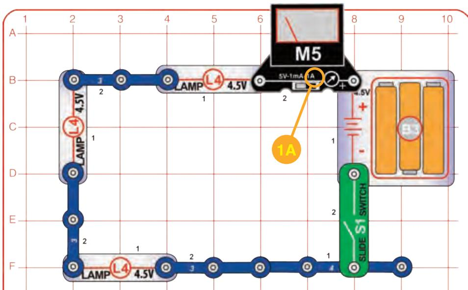
Build the main circuit and set the meter (M5) on the 1A setting. Turn on the slide switch (S1); the lamps (L4) light dimly and the meter (M5) measures the current through the circuit.
