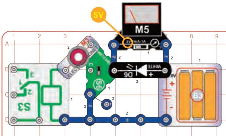
Build the circuit shown and set the meter (M5) to the 5V setting. Set the switcher (S6) to the bottom position; the meter shows that the full battery voltage is across the white LED (D6, and the LED is very bright.
