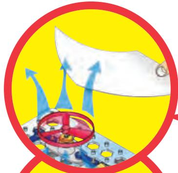
Build the circuit as shown, and set the switcher (S6) to the middle position at first, then set it to the bottom position to spin the fan. The fan blades suck in air around the motor (M1) and push it straight up. Hold a sheet of paper above the motor, it will get pushed up and away from the fan.
