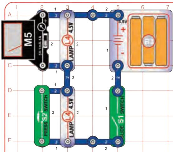
Build the circuit, and set the meter (M5) to the 5V setting. Turn on the slide switch (S1); the lamps (L4) are on and the meter measures the voltage across the top lamp. Push the press switch (S2) to turn off the bottom lamp.
