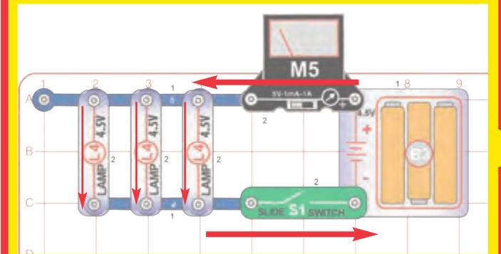
The three lamps are connected in parallel with one another. They are bright because each lamp gets the full battery voltage. The voltage pushes the current with equal force, because all are 4.5V, down each path.
