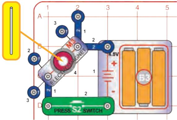
**Note:** the magnet poles may be opposite of how it's shown here, depending on how you connected the electromagnet (M3).
