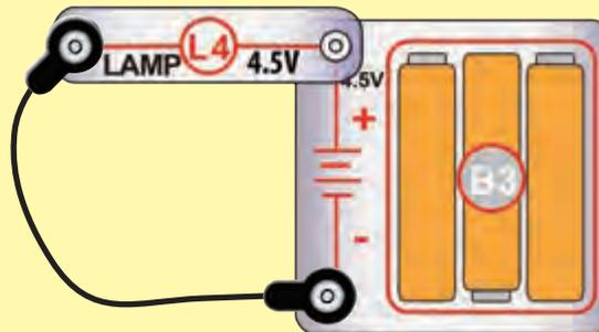
4. **Snap wires:** Use the mini-circuit below to test each of the snap wires, one at a time. The lamp should light.
