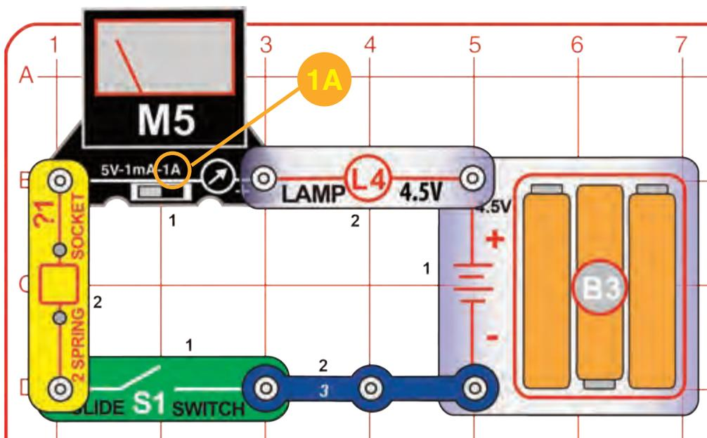
If you have the build-your-own electromagnet connected to the two-Spring socket (?1), disconnect its wires for this project. Build the circuit and set the meter (M5) to the 1A setting.
