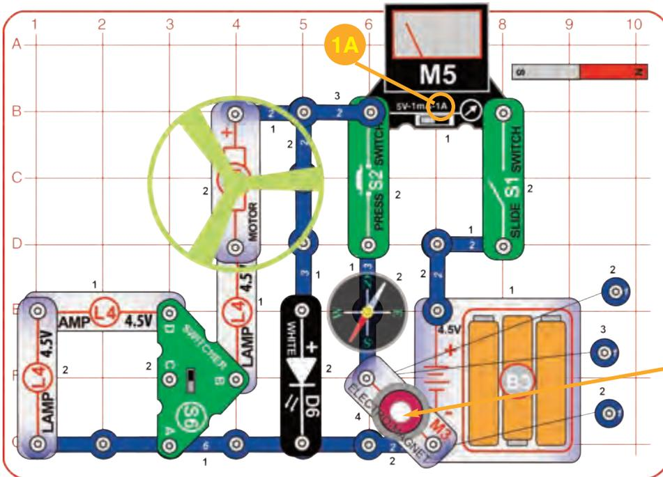
Build the circuit as shown, set the meter (M5) to the 1A setting, and place the magnet as shown. Turn on the slide switch (S1); the white LED (D6) lights and the meter measures the current. Set the switcher (S6) to the top position to make the fan spin, set it to the bottom position to make the fan spin faster, or set it to the middle position to turn off the fan. The compass is attached to the magnet; push the press switch (S2) to make the compass be attracted to the electromagnet (M3).
