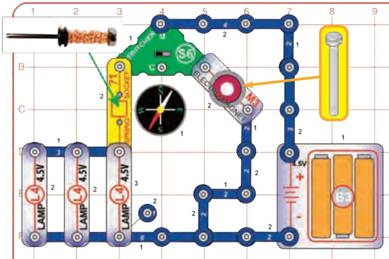
Assemble the build-your-own electromagnet (the thin wire wrapped around an iron core rod, with the ends connected to the 2-spring socket (?1)) using the instructions on page 5. Build the circuit, place the iron core rod in the electromagnet (M3).
