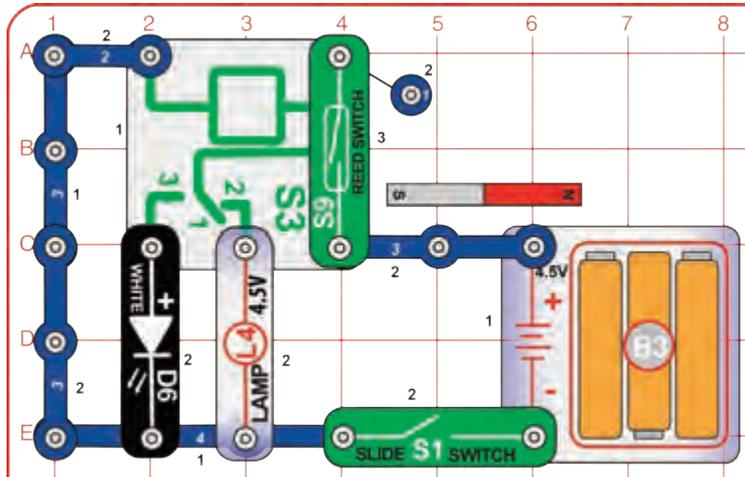
Build the circuit and turn on the slide switch (S1); the lamp (L4) should be on. Hold the magnet near the reed switch (S9) to activate the relay (S3), which turns the white LED (D6) on and the lamp off.
