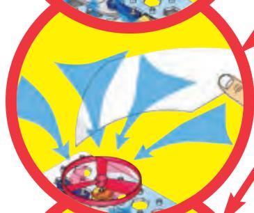
Flip the switcher to the top position now. The fan spins the other direction and sucks in air from above and pushes it down to the table. If the fan is spinning fast enough, then it will rise into the air when you turn off the switcher (sometimes it may fly off sooner due to vibrations). If you hold a sheet of paper near the motor, it will get sucked into the fan. If the fan doesn't fly off, then turn the switcher on and off several times rapidly when it is at full speed.
