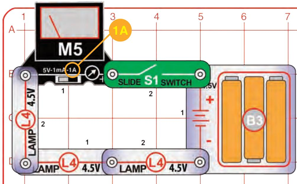
Build the circuit, set the meter to the 1A setting, and turn on the slide switch (S1). The three lamps (L4) are dimly lit, and the meter measures the current.
