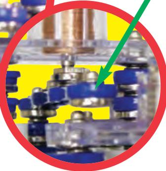
As in the preceding relay circuits, the current through the electromagnet makes a magnetic field that attracts the nut-snap, which breaks the circuit to the lamp. However in this circuit attracting the nut-snap also breaks the circuit to the electromagnet, which then releases the nut-snap. This creates a feedback loop which raises and releases the nut-snap in a repeating cycle. The buzzing sound you hear is from raising and releasing the nut-snap many times a second.
