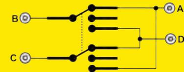
The switcher is used to reverse the battery connections (from snap A & D) to snaps B & C, which reverses the voltage across the motor and lamp. In the top position, battery "+" is connected to snap B, and in the bottom position battery "+" is connected to snap C.
