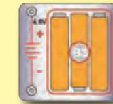
1. The batteries (B3) convert chemical energy into electrical energy and "push" it through the circuit, just like the electricity from your power company. A battery pushes electricity through a circuit just like a pump pushes water through a pipe.
