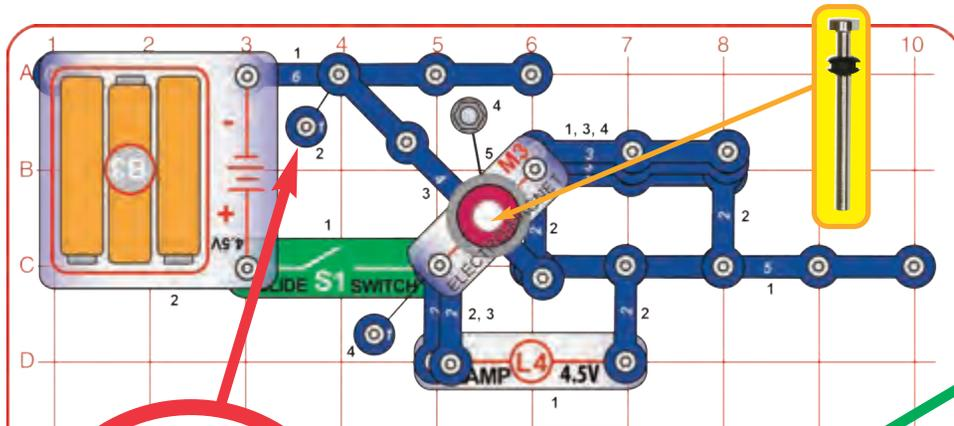
Build the circuit shown. At base grid location B6-B8, 3-snaps are on levels 1, 3 and 4. Snap the 4-snap onto the 1-snap at A4, then place it so it lays on the snap at C6 (DO NOT SNAP IT ON). Snap the nut-snap on the 4-snap so it will be under the electromagnet (M3). This circuit works best with new alkaline batteries.
