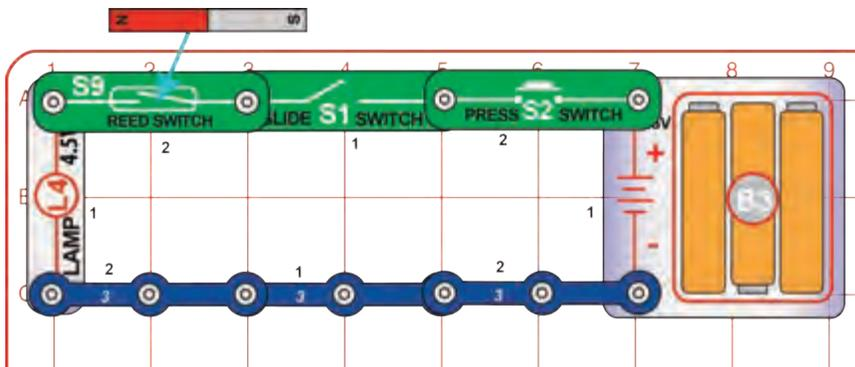
Place the magnet next to the reed switch (S9) to turn it on, push the press switch (S2), and turn on the slide switch (S1) in different combinations while seeing if the lamp (L4) lights. Fill out this table with the results:
