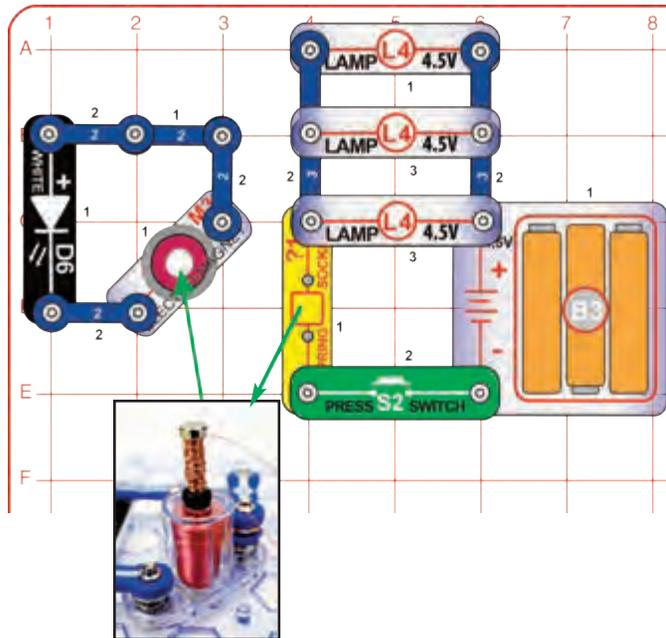
Build the circuit as shown. Assemble the build-your-own electromagnet as per the instructions on page 5. Push the wire on the build-your-own electromagnet to one side and insert its iron rod into the top of the electromagnet (M3), as shown.
