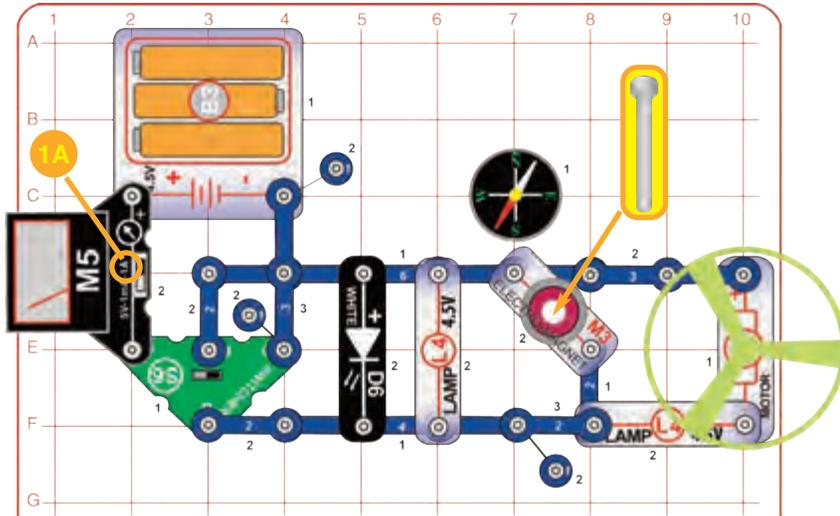
Build the circuit, set the meter (M5) to the 1A setting, place the iron core rod in the electromagnet (M3), and place the fan on the motor (M1). Set the switcher (S6) to the left or right to make electricity flow through the lights, motor, and electromagnet in opposite directions. The compass measures the magnetic field from the electromagnet and the meter measures the current from the batteries. Set the switcher to the middle position to shut off the circuit.
