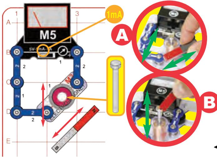
Build the circuit as shown. Place the iron core rod into the electromagnet (M3) and set the meter (M5) to the 1mA scale.
