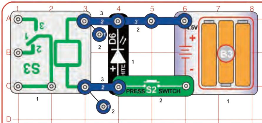
Build the circuit, then push and release the press switch (S2) while watching the white LED (D6).
