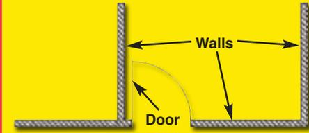
The electronics symbol for a simple slide switch should be thought of as a door to a circuit, which swings open when the switch is off. The "door" to the circuit is closed when the switch is on. This is shown here:
