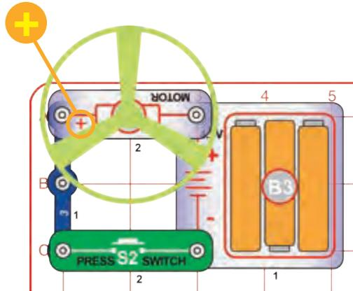
Build the circuit as shown and place the fan on the motor (M1). Be sure the "+" side of the motor is on the left.
