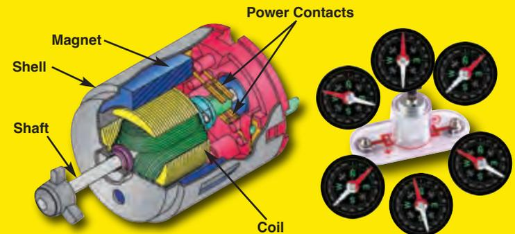
To prove the motor has a magnet inside, move your compass around it. The red needle will be attracted to one side but repelled from the other.
