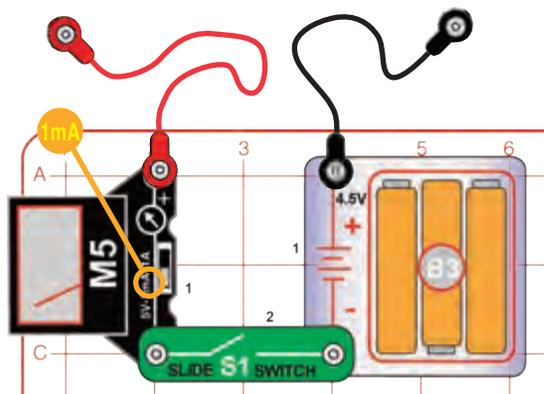
You can use Ohm's Law to measure the resistance of your puddles and drawings. The voltage is about 4.5V, and use the current measured on the meter.
