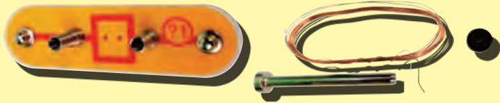
Wrap the coil around one of the iron core rods, leaving about 3 inches free at both ends. Place a grommet on the end of the rod to help keep the coil wire from coming off it.
