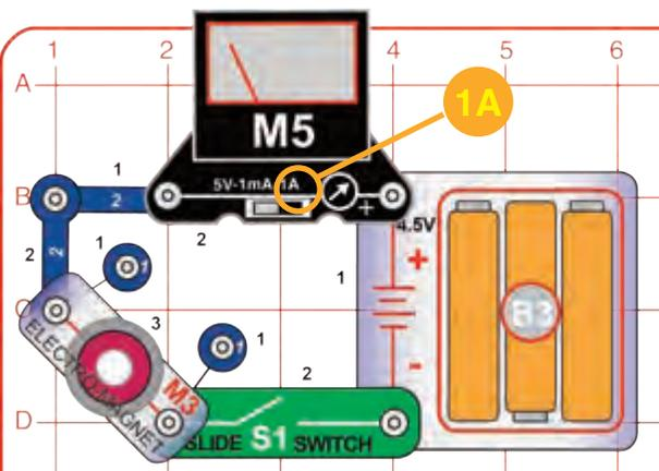
Build the circuit, set the meter (M5) to the 1A setting, and turn on the slide switch (S1). The meter measures the current through the electromagnet. Drop the thin rod into the electromagnet; it will be suspended in mid-air.
