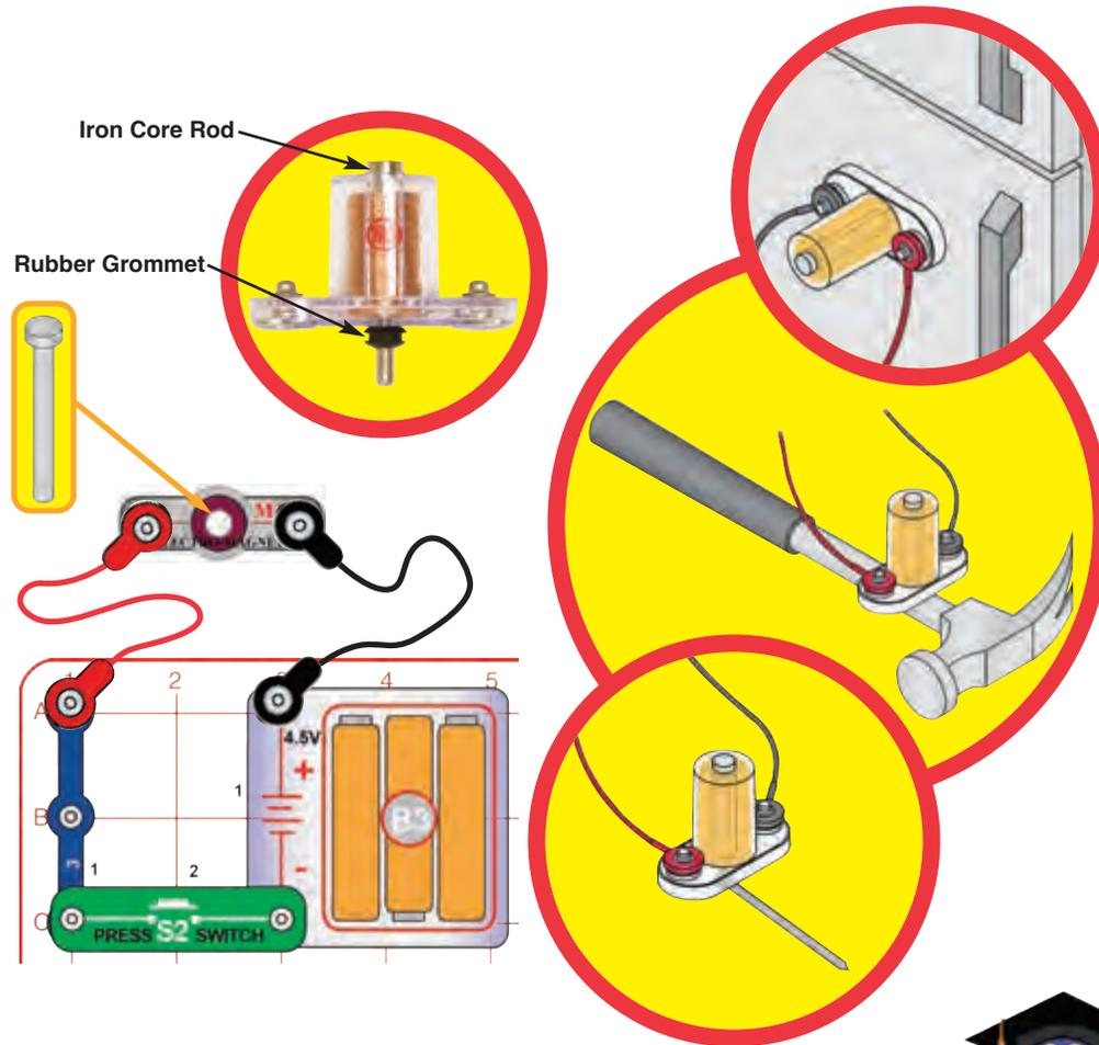
Build the circuit shown. Place the iron core rod inside the electromagnet (M3) and secure it with the rubber grommet. This project works best if you have new alkaline batteries.
