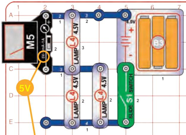
This circuit is like the preceding one, but adds a meter so you can compare the voltages across the lamps. Build the circuit, set the meter (M5) to the 5V setting, and turn on the slide switch (S1). The meter measures the voltage across the top lamp, which is bright.
