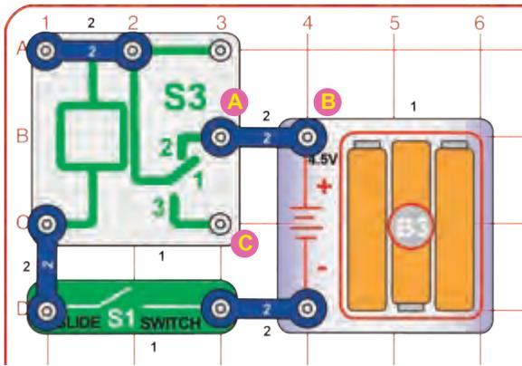
Build the circuit and turn on the slide switch (S1). The relay (S3) makes a buzzing sound.
