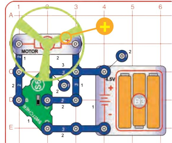
How does electricity turn the shaft in the motor? The answer is magnetism. The motor is the opposite of an electromagnet. Moving a magnet near a coil of wire can make a current flow in it (like the electromagnet), but a current flowing can move a magnet.
