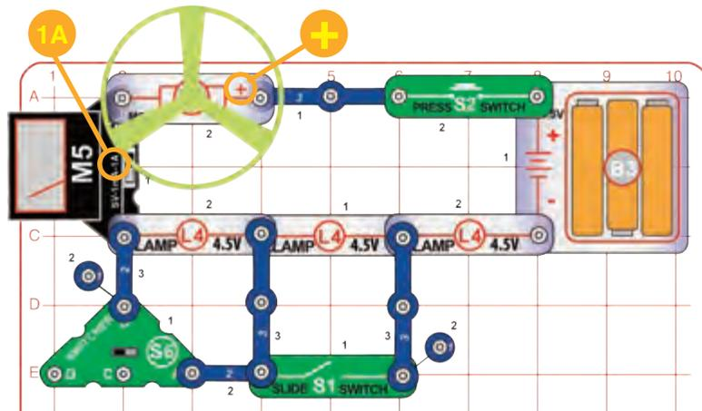
Build the circuit, set the switcher (S6) to the middle position (off), set the meter (M5) to the 1A setting, and place the fan on the motor (M1). Push switch (S2); the motor spins, and the meter measures the current. Turn on the slide switch (S1) or set the switcher to the right position to adjust the motor speed. You may need to give the motor a push to get it started, but do not touch it while it is spinning. Sometimes the lamps may not light.
