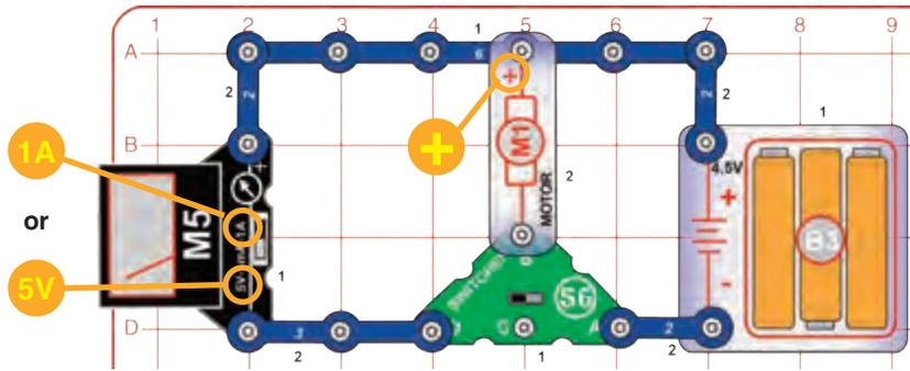
This circuit uses the batteries (B3) to get the motor spinning, then disconnects the batteries and uses the motor as a generator. A **generator** uses mechanical motion (here the spinning motor shaft) to create electricity (a current in a coil in the motor). The meter shows how much current and voltage are produced by the spinning shaft, with and without the fan.
