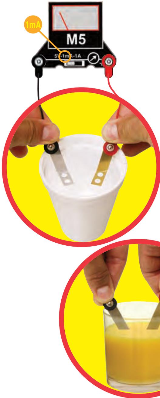
Set the meter (M5) to the 1mA scale and connect the jumper wires to it. Connect the other ends of the jumper wires to the snap electrodes (red to copper), and place them in a cup of water.
