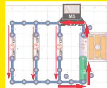
The current from the batteries splits up between the three lamps, because they are connected in parallel. Connecting parts in parallel allows more current to flow, so it decreases the overall circuit resistance.
