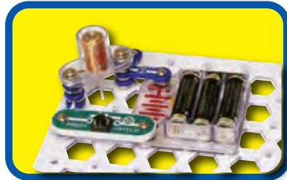
Build the circuit as shown and drop the thin rod into the electromagnet (M3). Push the press switch (S2) several times. The thin rod gets sucked into the electromagnet and can be suspended there, or you can bounce it up and down.
