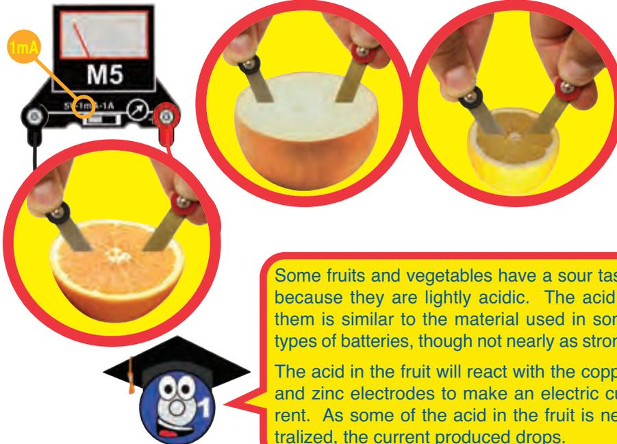
Some fruits and vegetables have a sour taste because they are lightly acidic. The acid in them is similar to the material used in some types of batteries, though not nearly as strong.
