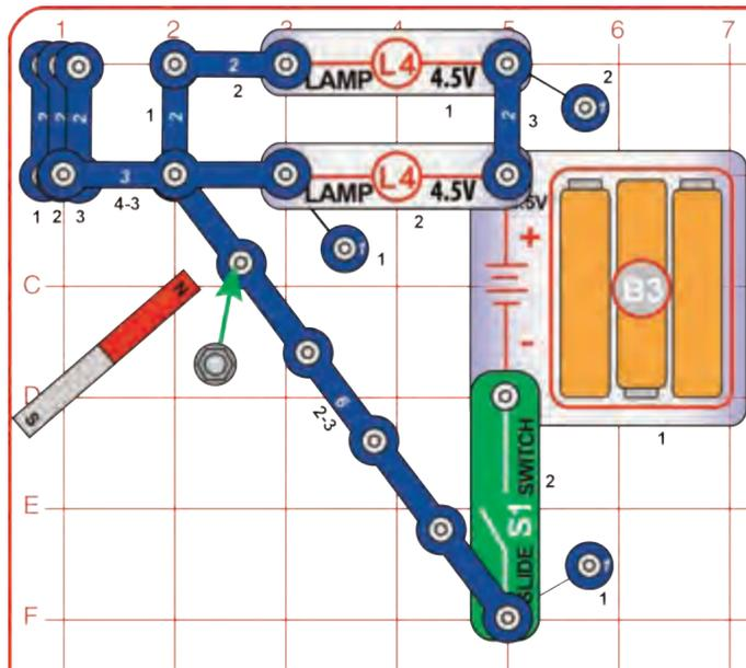
Build the circuit as shown. There are three 2-snap wires at base grid locations A1-B1. Snap the 6-snap wire at base grid location F5, then place it so it lays on the snap at grid location B2 (DO NOT SNAP IT ON). A 3-snap wire is placed across grid locations B1-B3, with the left side on lever 4 and the right side on level 3; sure it is securely snapped. Place the nut snap on the 6-snap wire.
