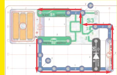
With the press switch on, current flows through a coil in the relay, which magnetically switches the relay's contacts. Now the relay's 1 and 3 contacts are connected, and current instead flows through the white LED.
