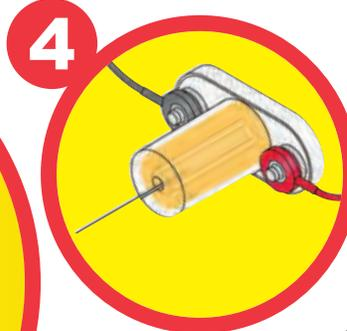
1. Use the circuit from the preceding project, with the iron core rod in the electromagnet (M3). An electronic magnet has a magnetic field just like an ordinary magnet. Hold your compass next to the electromagnet and push the press switch (S2). Move the compass all around the electromagnet and watch where the compass points.
