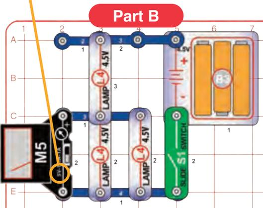
The resistance of the lower lamps is typically about triple that of the top lamp, but your results may vary. All wires have higher resistance when they are very hot.
