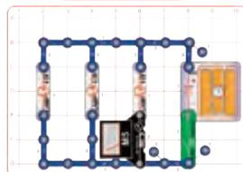
**Part C:** Swap the "B" location of the meter with the "C" 3-snap. The meter shows the current through circuit branch "C".
