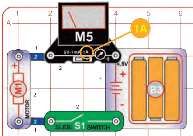
Build the circuit, set the meter (M5) to the 1A setting, and turn on the slide switch (S1). The motor (M1) spins and the meter measures the current. Do this with and without the fan on the motor.
