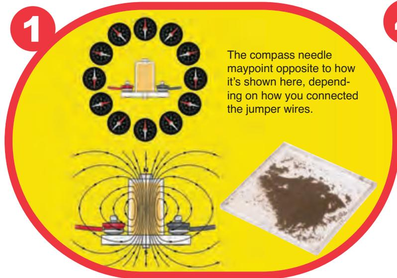
The compass needle may point opposite to how it's shown here, depending on how you connected the jumper wires.
