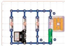
**Part B:** Swap the location of the meter with the 3-snap wire marked "B" ("+" side towards the lamp). The meter shows the current through circuit branch "B".
