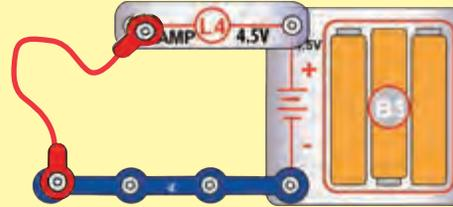
5. **Two-spring socket (?1) and coil (the build-your-own electromagnet):** use the mini-circuit in test step 4 but replace the 4-snap wire with ?1, with the coil connected between its springs; the lamp should light. If the lamp does not light be sure the protective coating has been removed from the ends of the coil wire where it attaches to the springs; if necessary use sandpaper or steel wool to scrape off the protective coating at each end.
