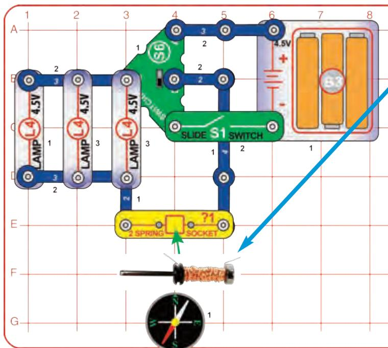
The wire magnet in the preceding circuit is not very powerful because it only has a few loops of wire, but you can make a better one. Assemble the build-your-own electromagnet (the thin wire wrapped around an iron core rod, with the ends connected to the 2-spring socket (?1)) using the instructions on page 5.
