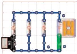
**Part A:** Build the main circuit, and set the meter (M5) to the 1A setting. Turn on the slide switch (S1); the lamps (L4) are all bright and the meter measures the current through the circuit.
