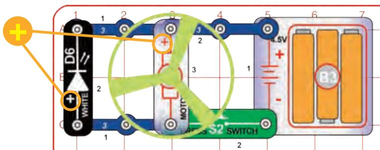
Build the circuit shown and watch the white LED (D6) as you push and release the press switch (S2). Notice that even though the LED is connected backwards, it is flashing dimly while the fan is spinning, and then flashes brightly when you release the press switch.
