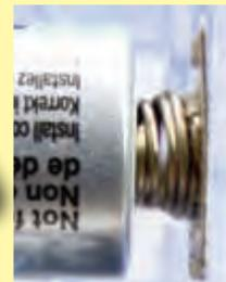
When installing a battery, be sure the spring is compressed straight back, and not bent up, down, or to one side.
