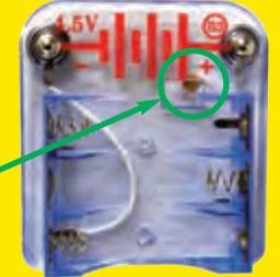
Fuses are designed to shut down a circuit when the current is abnormally high (indicating something is wrong, such as a component failure, bad design, or a person using it improperly). This shutdown prevents further damage to the circuit, and can prevent explosions or fires. Fuses are important for safety and most electrical products have one, especially if they use electricity supplied by your local electric company.
