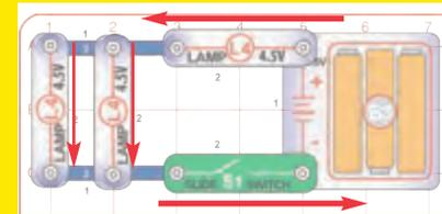
All the electric current flows through the right lamp, then divides between the two lamps on the left. The right lamp is much brighter than the others because it has twice as much electricity flowing through it, but that is not the only reason for the difference in brightness.
