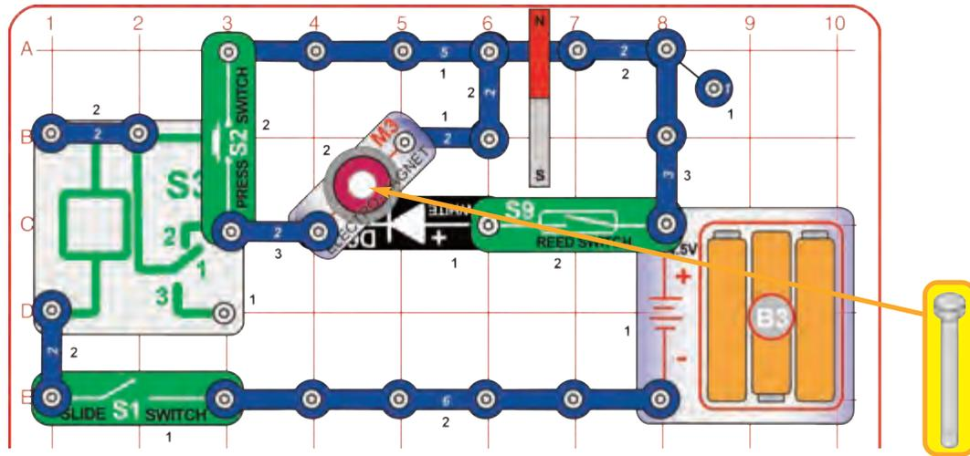
Build the circuit as shown, and turn on the slide switch (S1); you may hear a buzzing sound as the relay (S3) turns on and off rapidly. Adjust the sound by pushing the press switch (S3), raising and lowering the iron core rod in the electromagnet (M3), or by placing the magnet near the reed switch (S9) to activate it and the white LED (D6); try combinations of these and see how the sound changes.
