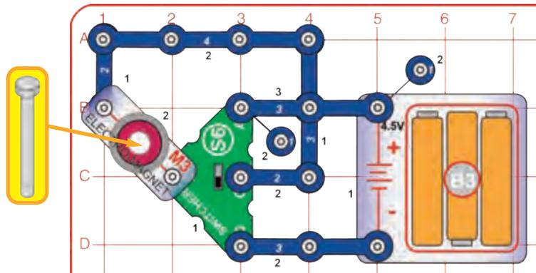
Build the circuit shown and place the iron core rod in the electromagnet (M3). Tie the magnet to a string and hold it just above the electromagnet, so that the magnet is attracted to the iron core rod without touching it. Flip the switcher (S6) back and forth between its top and bottom positions to reverse the electromagnet's magnetic field; the magnet flip around each time.
