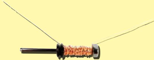
Check that some of the protective coating has been removed at each end, leaving about half an inch of bare wire. If the coil wire is broken (or later gets broken) then use sandpaper or steel wool to scrape off the protective coating for about half an inch at each end.
