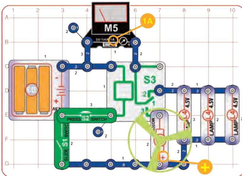
Build the circuit, place the glow fan on the motor (M1), and set the meter (M5) to the 1A setting. Turn on the slide switch (S1); the three lamps (L4) light and the meter measures the current.
