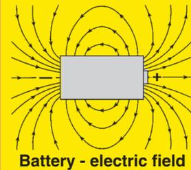
A magnet has a magnetic field, and a battery has an electric field. The north and south poles of a magnet are comparable to the positive and negative terminals of a battery.
