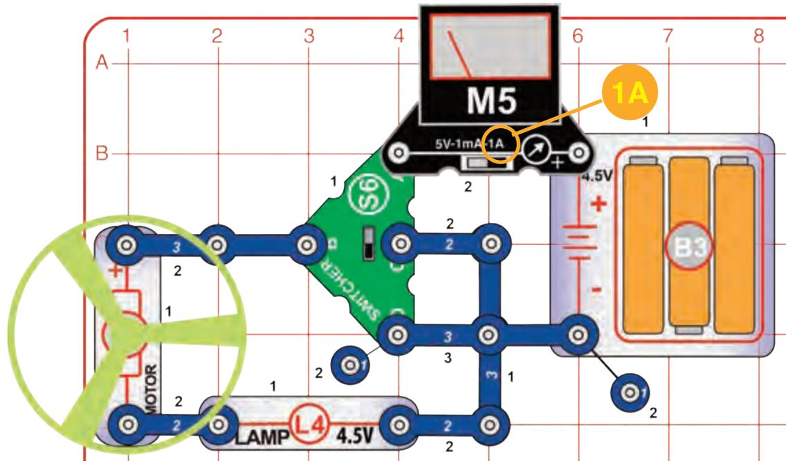
Build the circuit. Set the switcher (S6) to the middle position (off), set the meter (M5) to the 1A setting, and place the fan on the motor (M1). Now set the switcher to the top position; the motor spins, the lamp (L4) lights, and the meter measures the current. Set the switcher back to the middle position to turn off the circuit.
