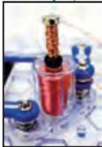
The buzzing sound produced by the relay is used to create a constantly changing magnetic field in the build-your-own electromagnet, which induces a current in the M3 electromagnet, which is seen on the LED and meter.
