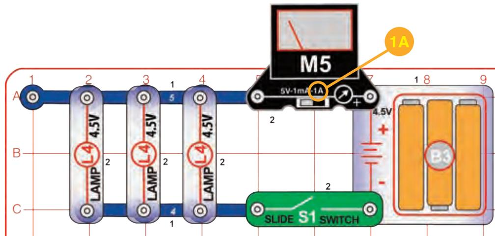
Build the circuit, set the meter (M5) to the 1A setting, and turn on the slide switch (S1). The lamps (L4) are bright and the meter measures the current.
