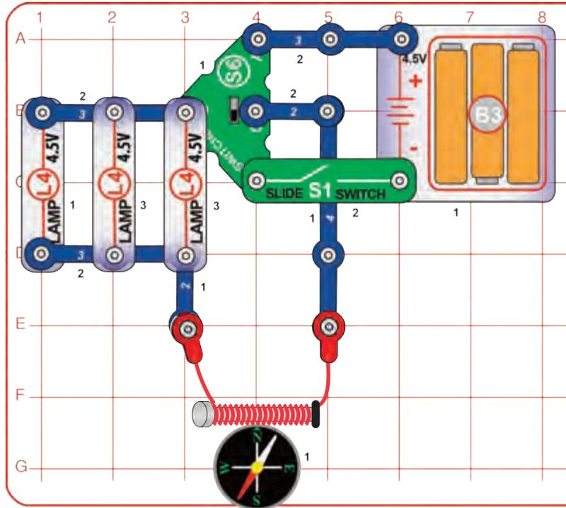
Build the circuit. Place the rubber grommet on one end of the iron core rod and wrap the red jumper wire tightly around it, as shown. Connect the red jumper wire to the circuit.
