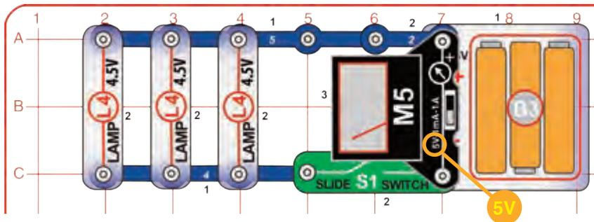
Build the circuit, set the meter (M5) to the 5V setting, but leave the slide switch (S1) off. The meter measures the voltage on the batteries. The lamps (L4) will be off, because the switch is off.
