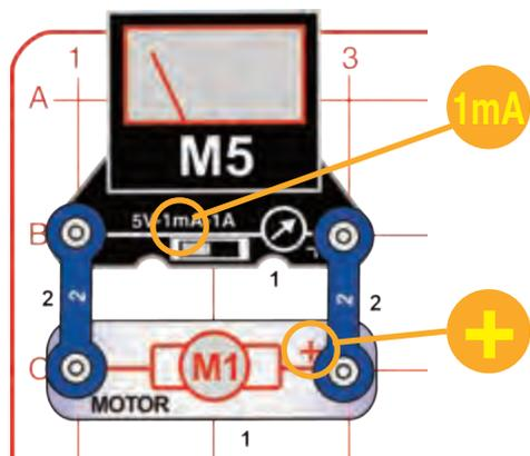
Build the circuit and set the meter (M5) to the 1mA scale. Spin the motor (M1) top clockwise with your fingers and watch how much current is produced. (Clockwise means in the direction in which the hands of a clock rotate.)
