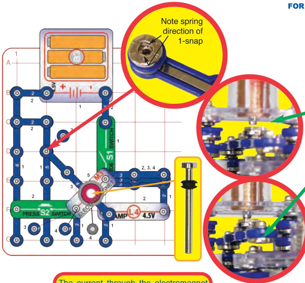
Build the circuit shown. Three 3-snaps are stacked together at base grid location E4-E6. Snap the 4-snap onto the 1-snap at grid location D2, then place it so it lays on the snap at F4 (DO NOT SNAP IT ON). Place the nut-snap on the 4-snap so it will be under the electromagnet (M3). This circuit works best with new alkaline batteries.
