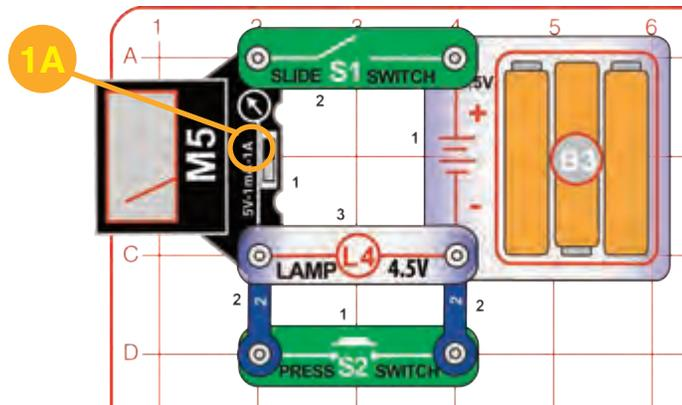
Build the circuit, set the meter (M5) to the 1A setting, and turn on the slide switch (S1). The lamp (L4) lights.
