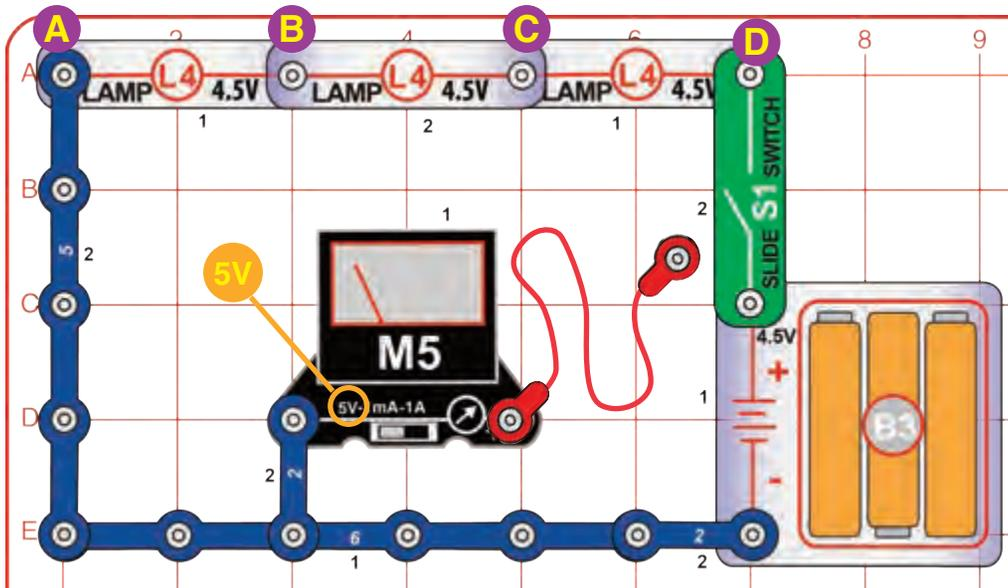
This circuit is similar to the preceding one, but measures the voltage instead of the current. Build the circuit, set the meter to the 5V setting, and turn on the slide switch (S1). The three lamps (L4) are dimly lit. Snap the loose end of the red jumper wire to points A, B, C, or D to measure the voltage at that point using the meter.
