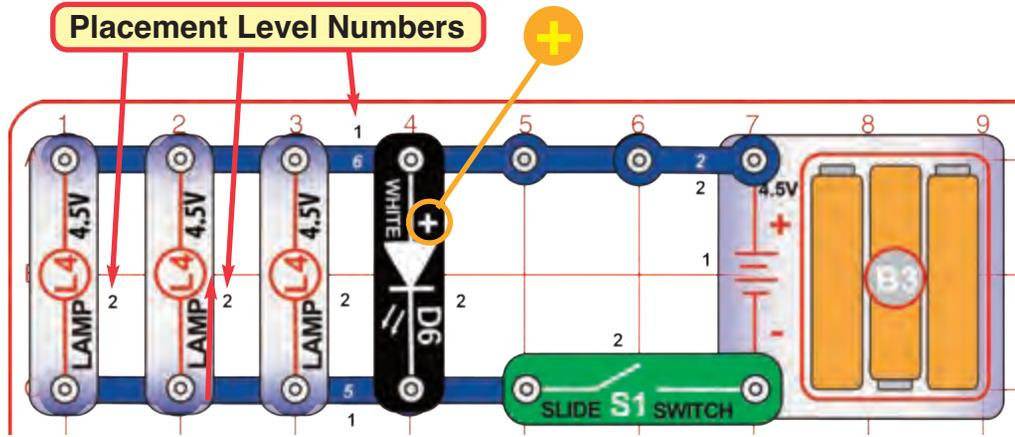
Build the circuit shown by placing all the parts with a black 1 next to them on the board first. Then, assemble parts marked with a 2. Install three (3) "AA" batteries (not included) into the battery holder (B3). Turn on the slide switch (S1); the lamps (L4) and white LED (D6) light.
