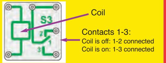
With the press switch off, the relay is off, so the 1 and 2 contacts are on the relay are connected, and current flows through the lamp.
