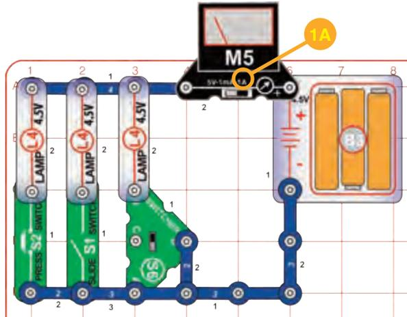
Build the main circuit, and set the meter (M5) to the 1A setting. Push the press switch (S2), turn on the slide switch (S1), or set the switcher to the top position (turning it on). Turn on the switches one at a time and in combinations, comparing the current on the meter.
