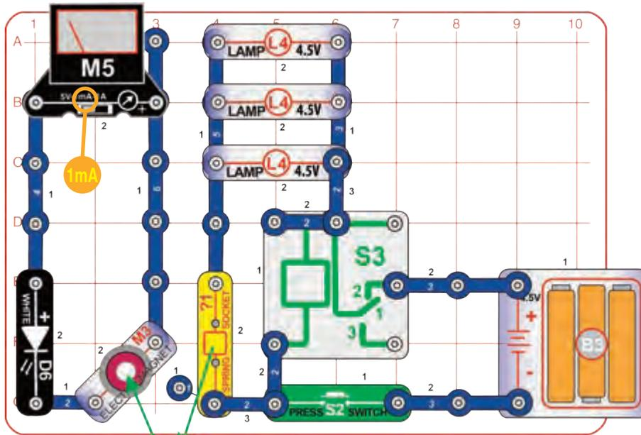
Build the circuit as shown. Assemble the build-your-own electromagnet as per the instructions on page 5. Push the wire on the build-your-own electromagnet to one side and insert its iron rod into the top of the electromagnet (M3), as shown. Set the meter (M5) to the 1mA setting.
