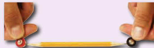
Build the circuit shown, and set the meter (M5) to the 1mA setting. Make your parts using either the water puddles method (A), the drawn parts method (B), or the pencil parts method (C), and turn on the slide switch (S1). Touch the metal in the jumper wires to your parts and read the current in milliamps.
