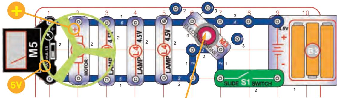
Build the circuit. Set the meter (M5) to the 5V scale, place the fan on the motor (M1), and drop the thin rod into the electromagnet (M3).
