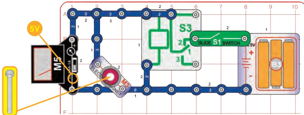
Build the circuit, set the meter (M5) to the 5V setting, and turn on the slide switch (S1); you hear a buzzing sound as the relay (S3) turns on and off rapidly. Adjust the sound by raising and lowering the iron core rod to different heights in the electromagnet (M3), to make music. The meter shows how the voltage is changing.
