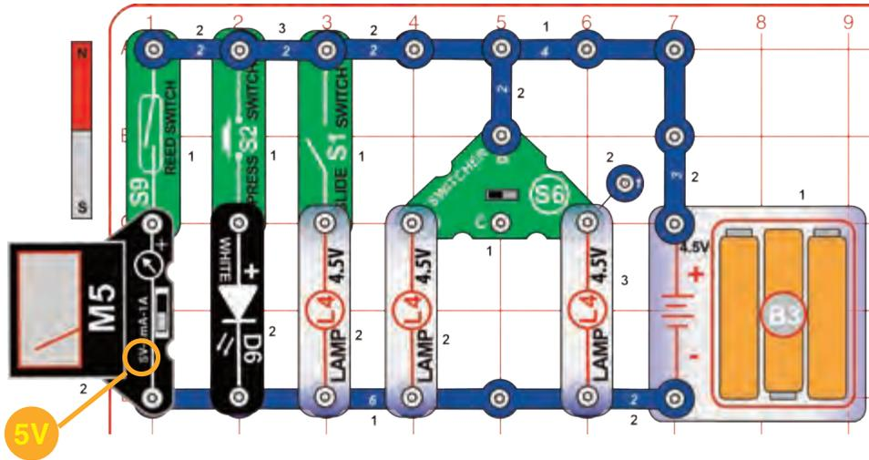
Build the circuit, set the meter (M5) to the 5V setting, and initially set the switcher (S6) to the middle position. Turn on each of the switches:
