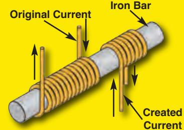
Transformers allow circuits to be isolated from each other, since the connection between them is magnetic and not electrical. Transformers can also change the voltage by using coils with more or less loops of wire.
