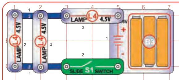
Build the circuit. Turn on the slide switch (S1) on and off several times, watching the brightness of each lamp (L4). Compare the brightness of each lamp, and how quickly each turns on.
