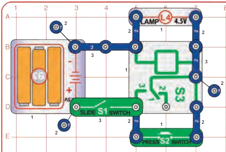
Build the circuit and turn on the slide switch (S1). Nothing happens. Now push the press switch (S2). The lamp (L4) comes on and stays on even after you release the press switch (the circuit “remembers” that you pushed the press switch). Turn off the slide switch to turn off the lamp.
