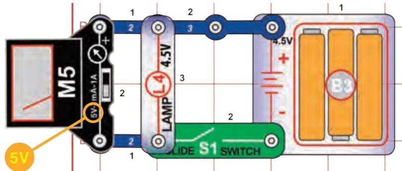
Build the circuit, set the meter (M5) to the 5V setting, and turn on the slide switch (S1). The lamp (L4) lights and the meter measures the voltage.
