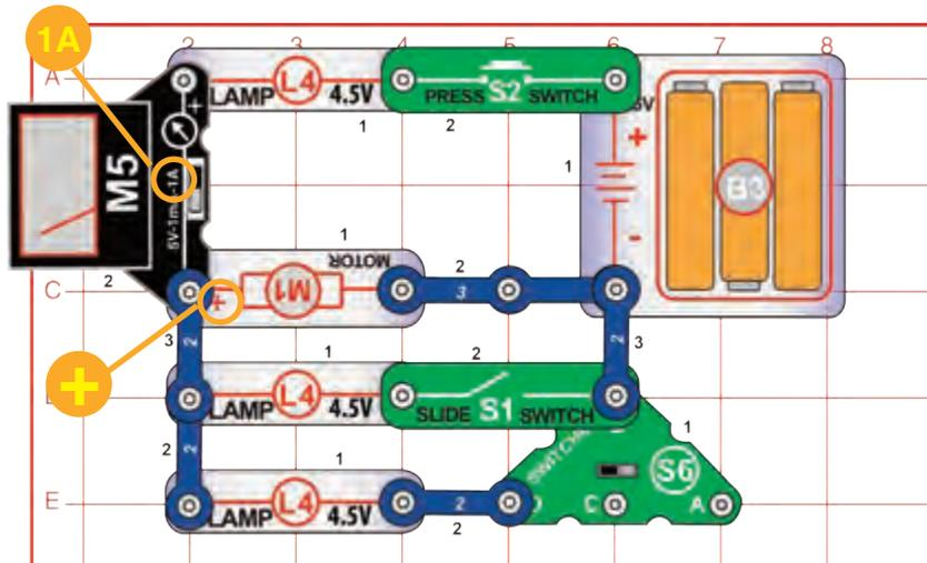
Build the circuit, set the switcher (S6) to the middle position (off), set the meter (M5) to the 1A setting, and leave the fan off the motor (M1). Push switch (S2); the motor spins, and the meter measures the current. Turn on the slide switch (S1) or set the switcher to the left position to adjust the motor speed. You may need to give the motor a push to get it started, but do not touch it while it is spinning. Sometimes the lamps may not light.
