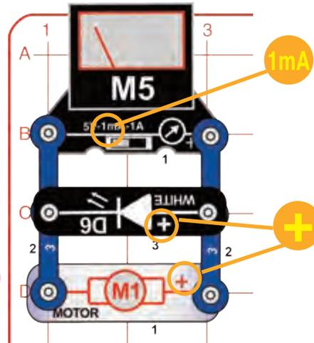
Build the circuit and set the meter (M5) to the 1mA scale. Using the string, make a small loop at one end and put it on a prong of the motor (M1) top. Wind a few feet of the string around the motor shaft (wind it so that pulling the string will spin the motor shaft clockwise).
