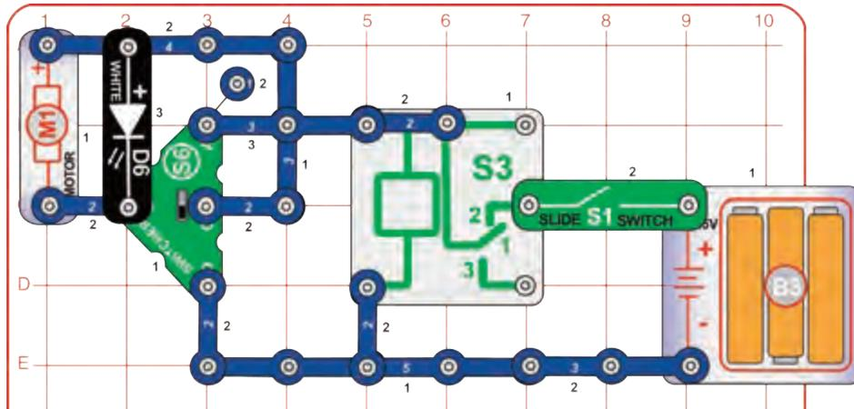
Build the circuit as shown (leave the fan off the motor), and turn on the slide switch (S1); you hear a buzzing sound as the relay (S3) turns on and off rapidly. Set the switcher (S6) to the top or bottom position to turn on the motor (M1) and white LED (D6).
