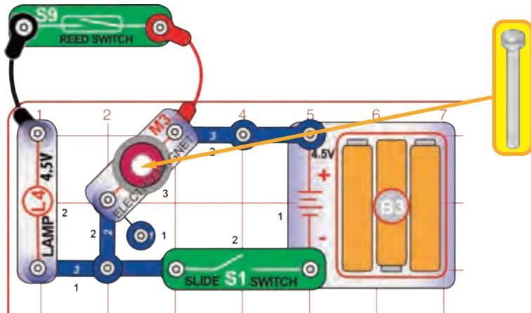
Build the circuit, place the iron core rod in the electromagnet (M3), and turn on the slide switch (S1). Use the red & black jumper wires to hold the reed switch (S9) over the electromagnet to turn on the lamp (L4). You can also activate the reed switch by holding the magnet close to it.
