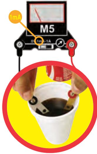
Set the meter (M5) to the 1mA scale and connect the jumper wires to it. Connect the other ends of the jumper wires to the snap electrodes (red to copper), and place them in a cup of cola soda.
