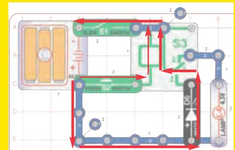
The current through the press switch activates the coil in the relay, which changes the relay connection from contacts 1-2 to contacts 1-3. There is no electrical connection between the relay's coil and 1-2-3 contacts, so those circuits do not affect each other, and can operate at different voltages. In this way a low-voltage circuit can control a high-voltage or high-current circuit.
