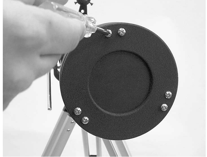
Figure 9. Loosen one screw on the back of the optical tube one full turn and tighten the other screw "in the set" until tight to adjust the primary mirror.
