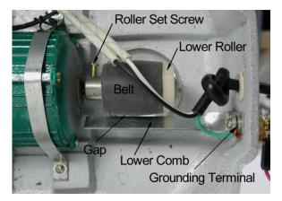
9. Unplug the generator and loosen the set screw that holds the lower roller on the
